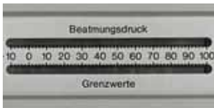
Airway pressure monitor on the UV-1 with depiction of limit values
